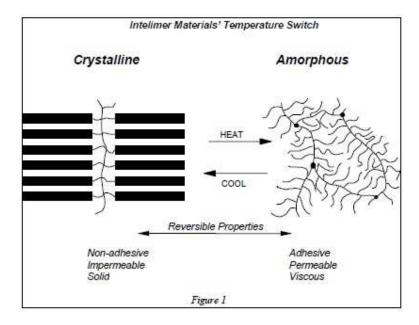
This chemical structure provides an additional benefit. Spatially distinct regions of the Intelimer polymer confer different physical properties on the material. Each part can be tuned independently to meet the needs of a given application. For example, the switching temperature (which arises from one part of the chain) can be adjusted independently of adhesive properties (which arise from another part of the chain).
